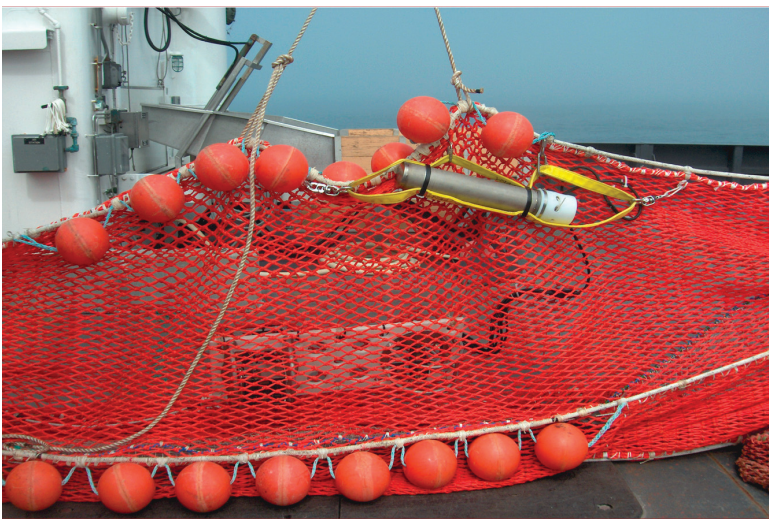
Figure 4. Sled and housing system mounted within a midwater trawl net to visually verify acoustic backscatter collected during the acoustic survey for hake.
