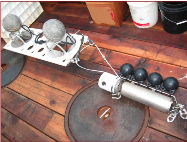
Figure 1. Two-part video camera and recording system
