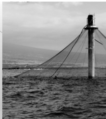
Figure 1. (Left) A typical offshore array of submersible cages—SeaStations from OceanSpar, Bainbridge Island, WA. The photo at right is a surfaced 6400 m 3 cage.
