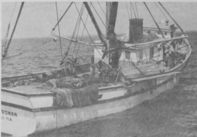
LARGE SHRIMP TRAWLER AND GEAR ARRANGED FOR SETTING
