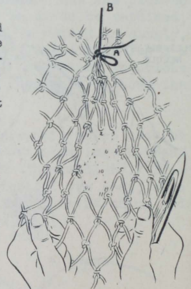
FIG. 18 - SUPPORTING DAMAGED NET
