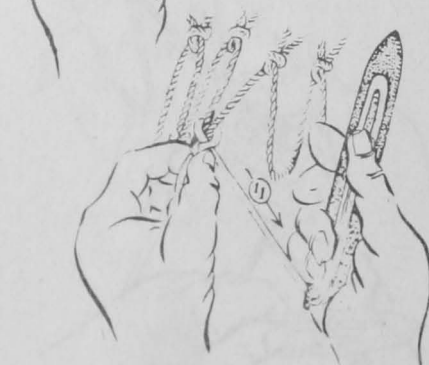
FIG. 25 - HALF-MESH KNOT L TO R WEAVING
