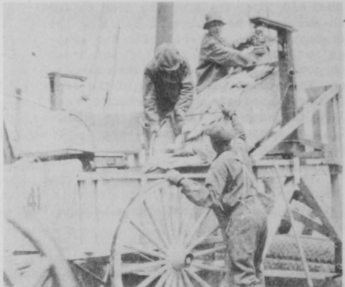
FIGURE 6 - A WEIGHING PLATFORM AND BOX WITH HINGED END FOR DISCHARGING FISH INTO CARTS.
