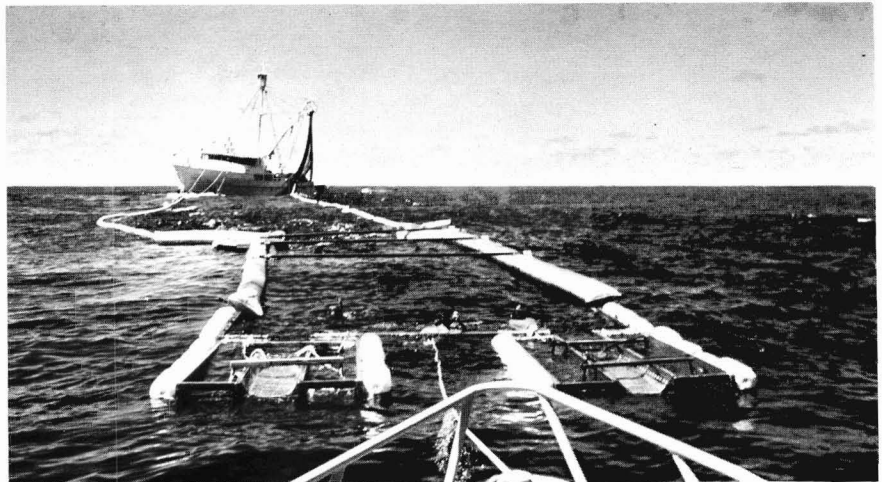
The Porpoise School Impoundment System in operation during a research cruise of the Cooperative Dedicated Vessel Program. Porpoise are being maneuvered from the tuna purse seine into the corral for examination and tagging.
