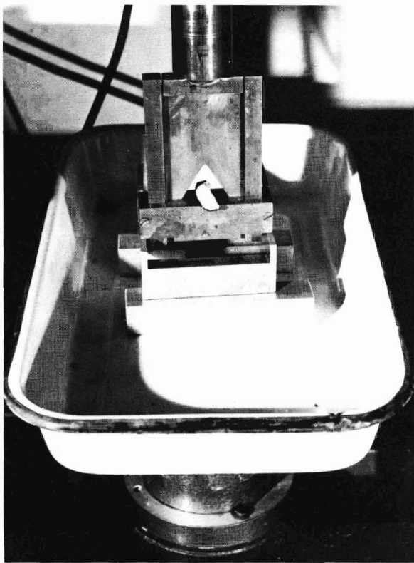
Figure 5.—Warner-Bratzler-type shear press and sample of blue shark flesh.
