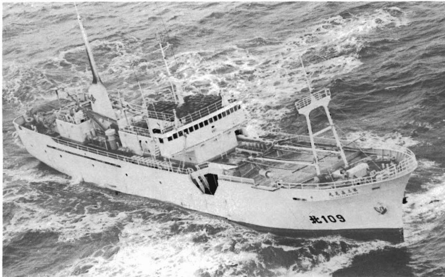
Figure 8.—Japanese longline-gillnet vessel, 55 m in length and 424 gross tons.
