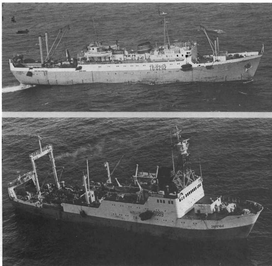
Figure 11.—Soviet factory stern trawlers: a large (BMRT) trawler of 3,170 gross tons (upper panel) and the newer type (RTM) trawler of 2,657 gross tons with greater deck space aft (lower panel).
