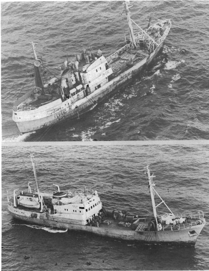
Figure 10.—Soviet medium side trawler of 500 gross tons (upper panel) and large side trawler of 700 gross tons (lower panel).
