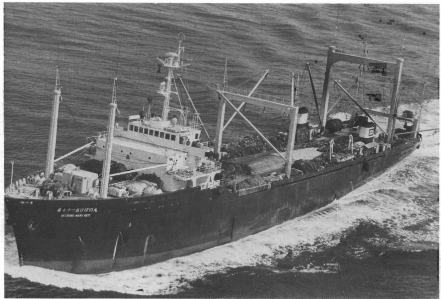
Figure 7.—Japanese large independent stern trawler, 100 m in length and 3,200 gross tons.
