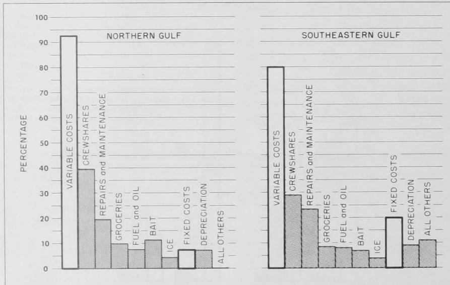
Figure 4.—Comparison of variable and fixed costs by type for large (56-69 feet) red snapper-grouper vessels operating in the northern and southeastern Gulf of Mexico, 1974 and 1975.
