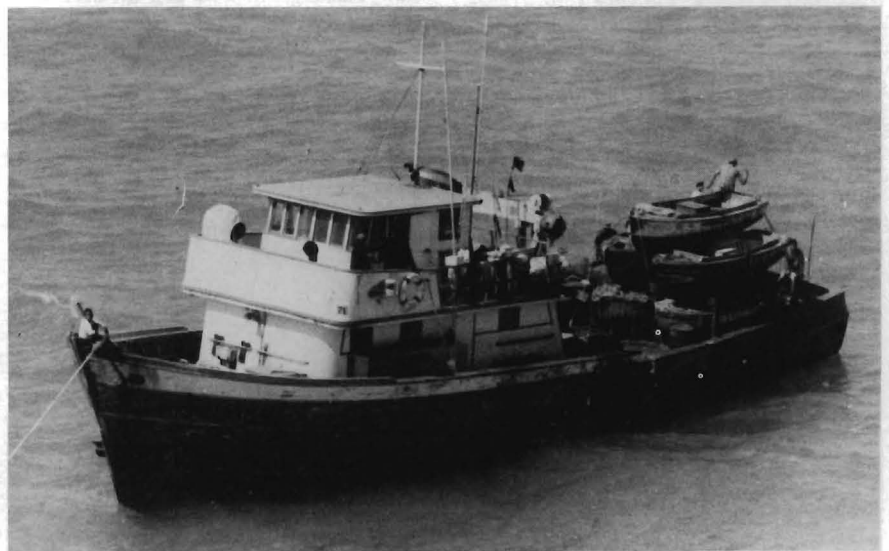
Figure 4.—The 75-foot (23-m) Lambda is the principal vessel used by the Cuban Gulf Fleet. Longlining launches can be seen stacked on the after deck. Photograph courtesy of the Law Enforcement and Marine Mammal Protection Division, NMFS, NOAA, St. Petersburg, FL. 33702.
