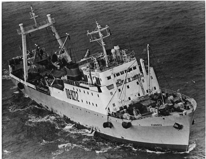
Figure 11.—Factory stern trawler Polevod of new RTM class. Vessels of the RTM class are somewhat smaller than BMRT's but have a larger deck area aft for handling gear and fish.
