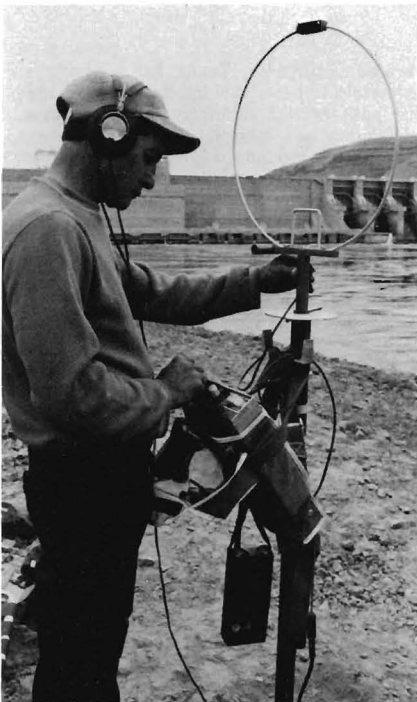
Figure 12.—A fish tracking team member taking a bearing on a radio-tagged salmon below Lower Monumental Dam. Simultaneous bearings taken by two or more team members will be used to establish the location of the fish by triangulation.
