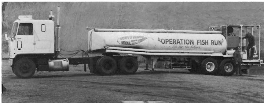
Figure 20.—Tank trucks transport fish from collection and marking area around the hazards of seven dams and six impoundments for release below Bonneville Dam, about 350 miles downstream from Little Goose Dam. Studies are also being carried out at Lower Granite Dam in which eight dams and seven impoundments are being bypassed.
