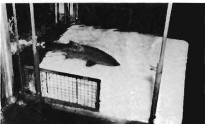
Figure 13.—Adult salmon passing over a white counting board which aids observer in identifying species.
