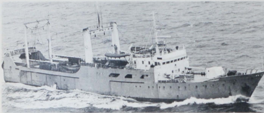
Figure 5.—The Republic of Korea's first high-seas stern trawler, the 1,330 GRT Kang Wha 601 , photographed off Alaska in 1969.
