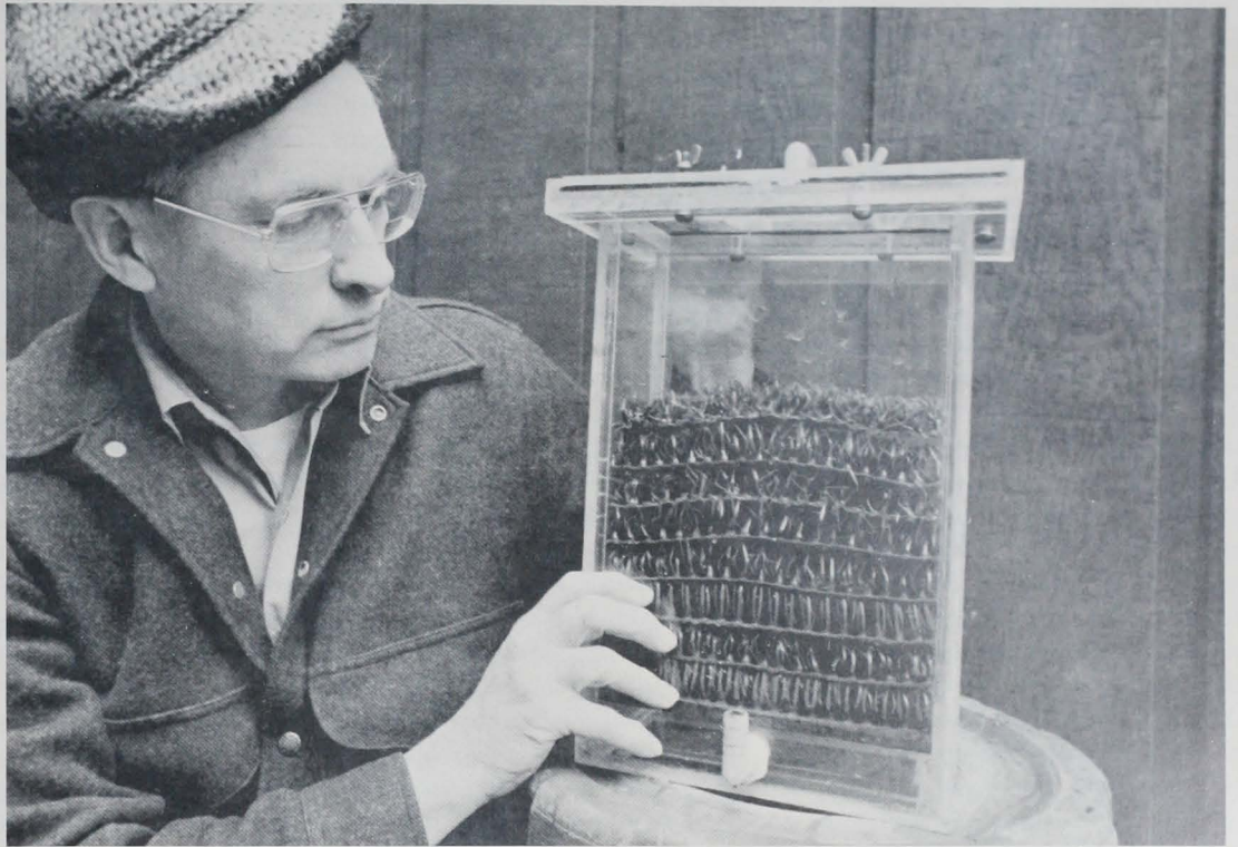
(Above) Pink salmon eggs were incubated to the emergent fry stage in this transparent box with eight layers of AstroTurf.
