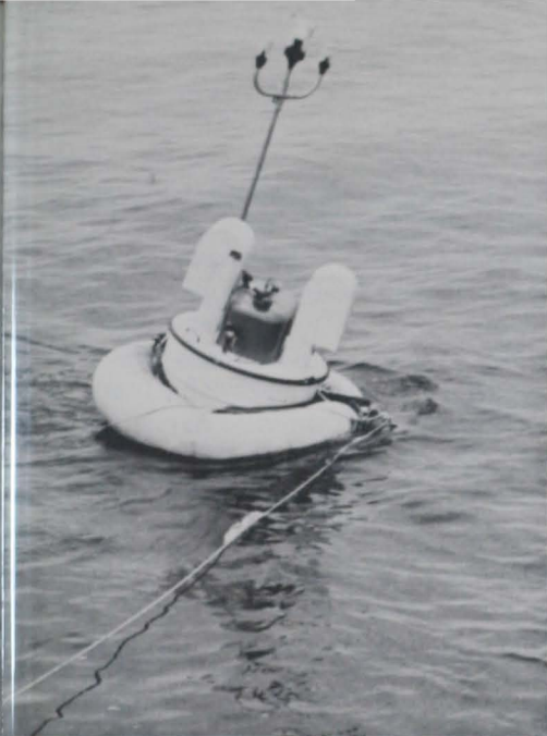
Figure 6.—The prototype FLAB unit anchored on station in a current greater than two knots.
