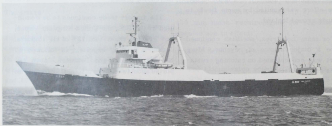
The 240-foot, all-freeze, over-the-stern-part factory trawler. Owned by Britain's Boston Deep Sea Fisheries Ltd.
