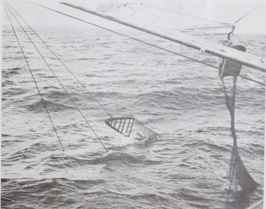
Fig. 6 - Doors submerged and sled about to submerge during trawl setting.
