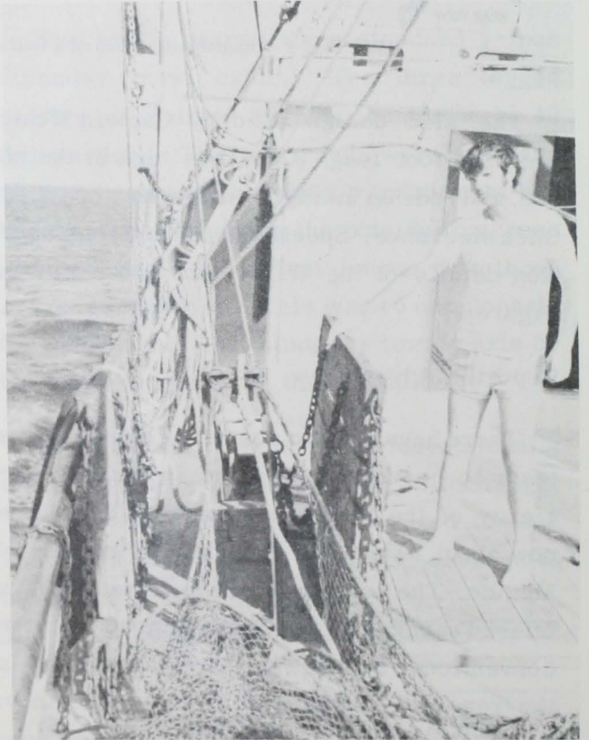
Fig. 4 - Aft view of sled and doors in position for pickup to outrigger boom.
