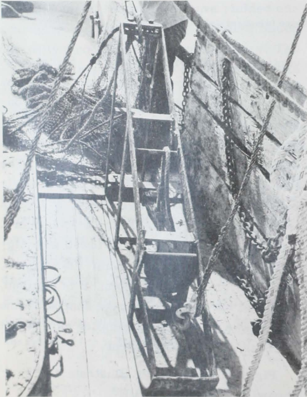
Fig. 3 - Front view of sled showing towing bridle and lazyline tag.
