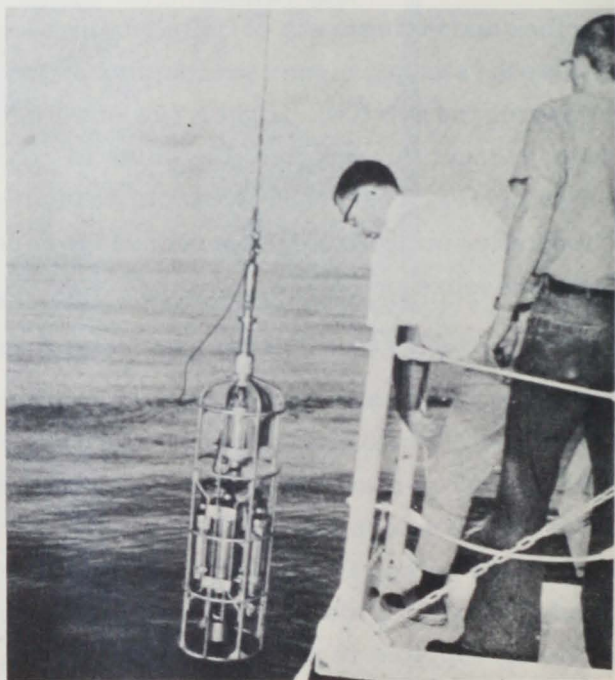
(Top) Readyng a plankton sampler. (Bottom) Multisensor package senses salinity, conductivity, temperature, and depth. It relays these measurements to electronic equipment in research ship's oceanographic laboratory.
