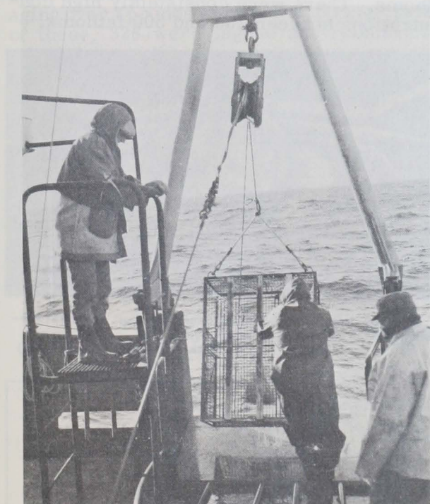
Fig. 4 - Lobster pot coming aboard Delaware II. Note movable gantry and track (at bottom).
