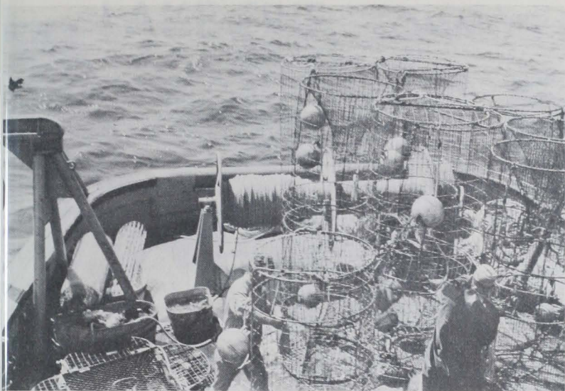
Fig. 1 - These pots on deck of John N. Cobb will be fished from a groundline.
