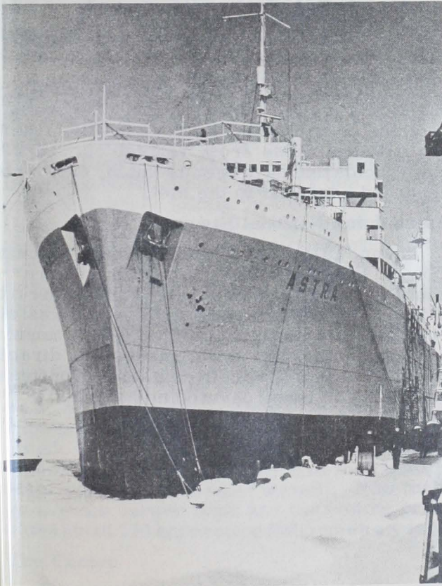
Fig. 1 - Motor/Ship 'Astra', a 25,000-ton, $7-million "floating factory" operated by Astra Nutrition of Sweden. It will process high-grade fish protein concentrate (FPC) from daily catch of fishing boats.
