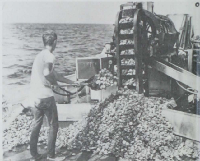
Fig. 5 - Feeding the bucket conveyor leading to "separator."
