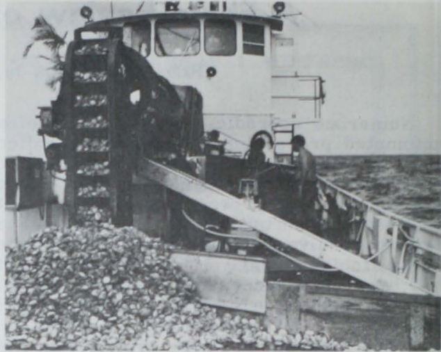
Fig. 4 - Overall view of main deck processing equipment. Includes conveyor "separator" with trash overboard trough, "shucker" with shell overboard trough, and salt-water "cleaning trough" to below-deck eviscerator.
