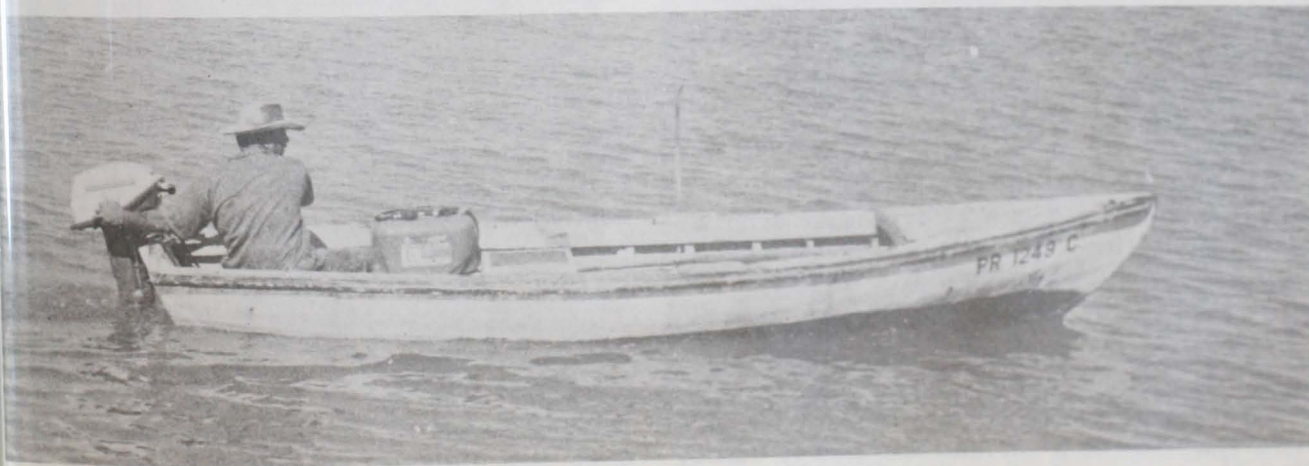
Fig. 5 - Sixteen-foot outboard motor fishing boat called "yola" is the most popular fishing craft.
