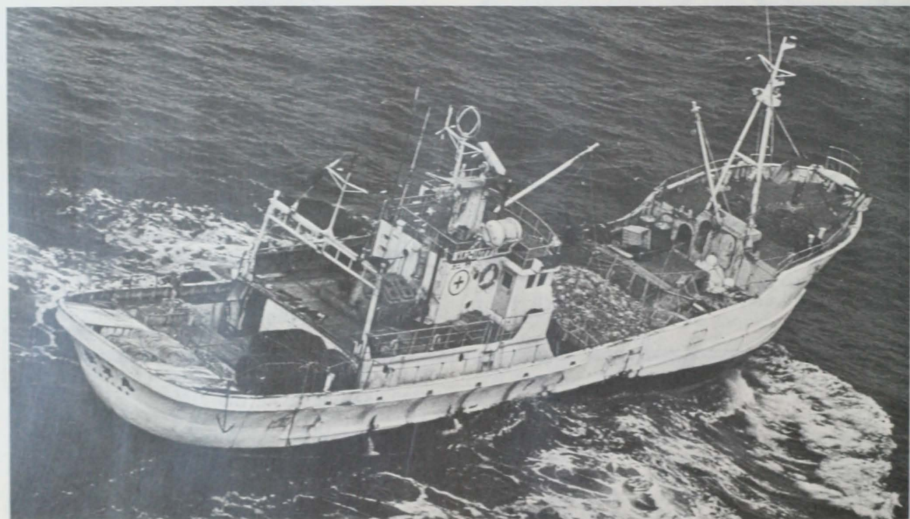
Fig. 3 - Aerial view of Japanese vessel handling tanner crab pots. Crab are visible stowed in sling loads on well deck. Longlines that carry the pots are coiled on fantail, with nested pots stored to one side.
