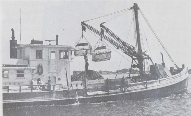
Fig. 6 - Transplanting boat partially loaded with seed oysters. Booms are used to lift dredges over the deck. After boat is loaded, seed oysters are washed overboard on growing beds by hosing with water under low pressure. Cost of transplanting seed oysters ranges from 4 to 10 cents per bushel.
