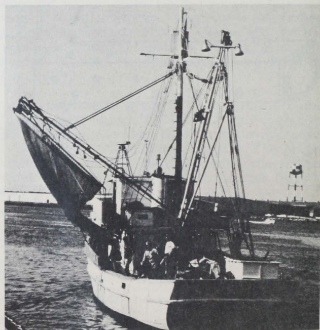
Fig. 5 - George M. Bowers departing on collection trip with 5-meter lift net suspended from port outrigger. The net hoop was attached to outrigger and yard arm (see Fig. 4) permitting lift lines to be slackened and outrigger raised to clear dock.
