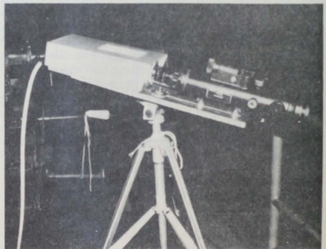
Fig. 3 - Starlight scope coupled to television camera.
