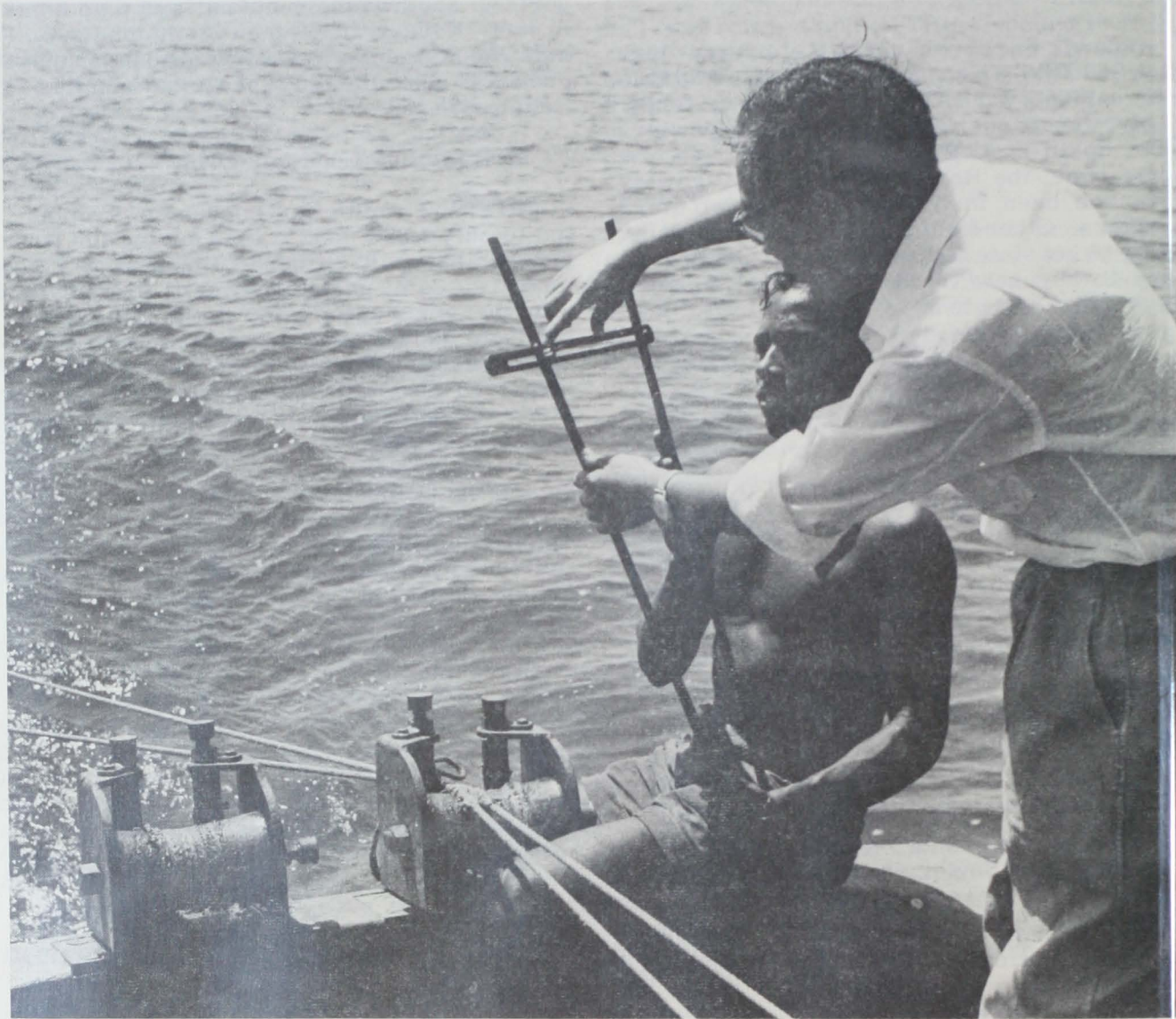
A Japanese expert working for FAO shows Indian fisherman how to measure opening of shrimp trawl. (FAO: S. Bunnag)
