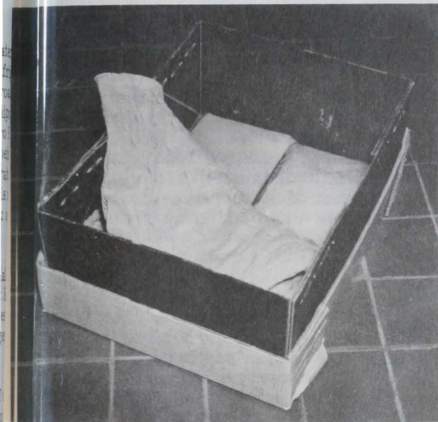
Fig. 1 - Modified Wet-Lok crab shipper prepared with gel-ice and Kimpak prior to prechilling.
