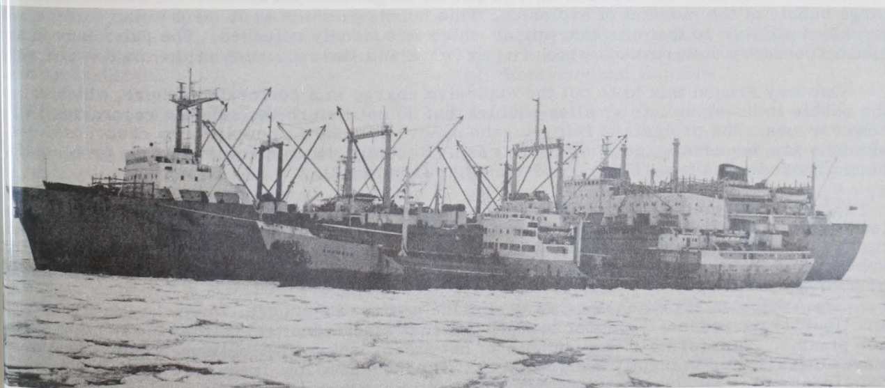
Fig. 3 - The 571-foot long Soviet base or factory ship 'Spassk' nested with a tanker (visible in picture) and a refrigerated transport, a stern trawler, and a tug (only masts shown in picture) in ice pack in central Bering Sea. These ships are part of the approximately 70-vessel winter herring expedition off Alaska. (J. Branson)
