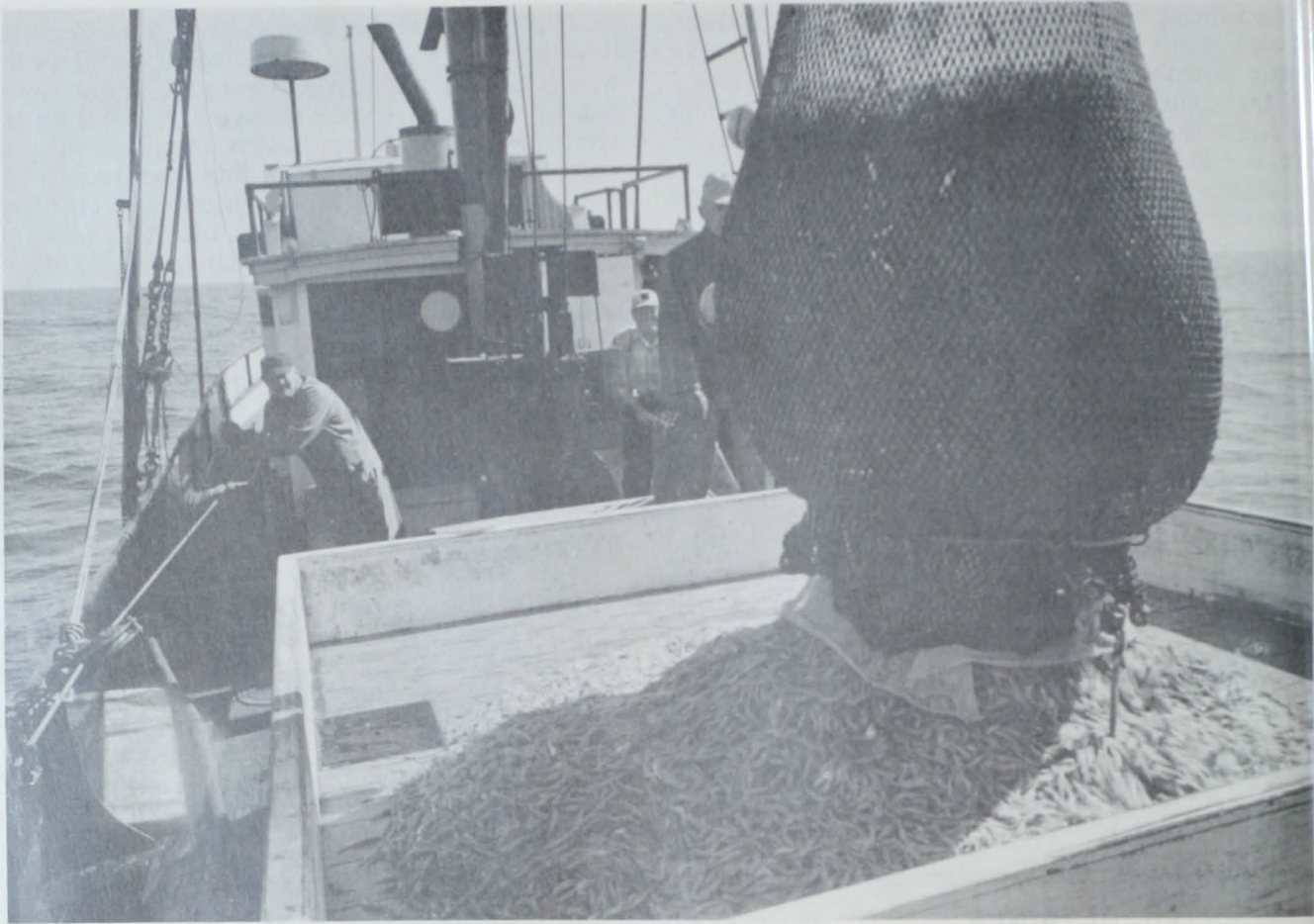
Fig. 7 - A nearly pure shrimp catch is dumped from a BCF shrimp sorting trawl onto the M/V Washington's sorting table. This 2,000-pound catch of shrimp had less than 20 pounds of smelt and flounders.
