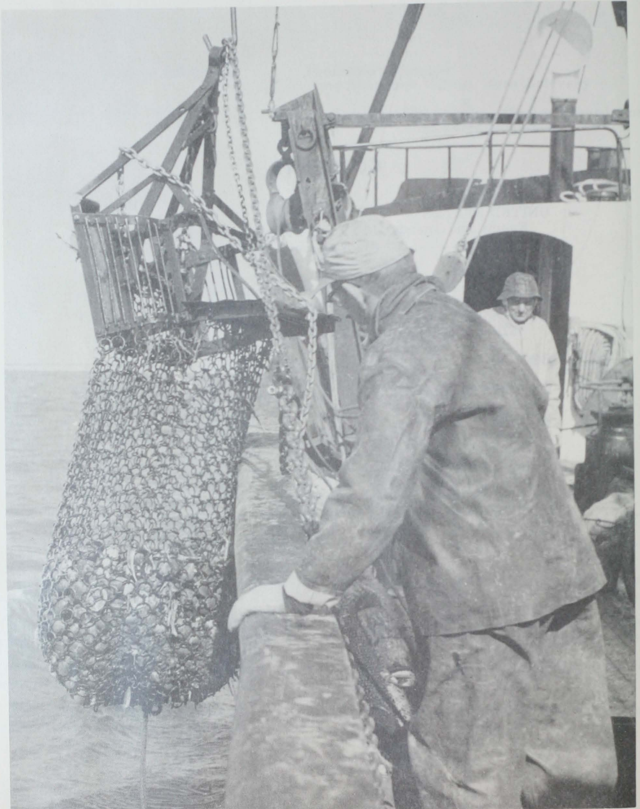
A 14-tooth 'Fall River' clam dredge rigged with an accumulator-chain modification--used for exploratory fishing by R/V 'Silver Bay' off North Carolina. (Photo: J. B. Rivers)
