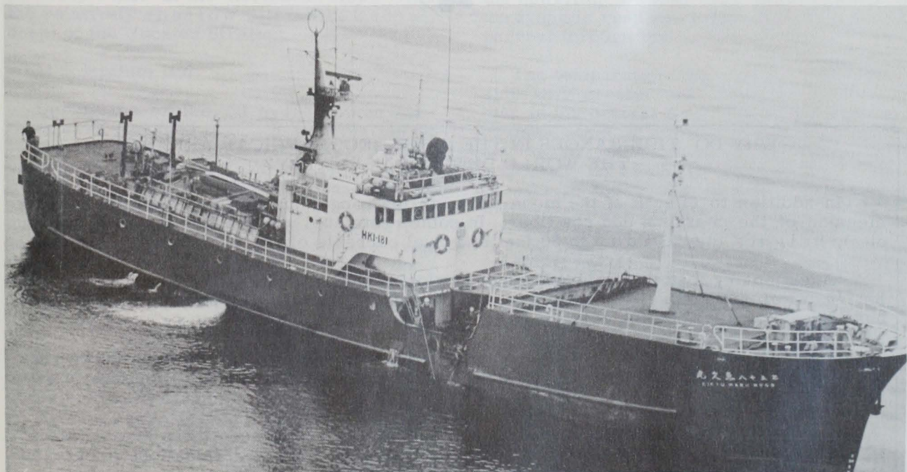
Fig. 9 - The 'Eikyu Maru #58' was built in 1967, primarily for the northern water longline fishery. Shelter over working area is permanent and part of original construction. Baiting and gear-setting areas are also enclosed in hull, rather than placed in temporary house on upper deck. The ship is 299 gross tons, 124 feet long, powered by a 700 hp. slow-speed diesel, and has crew of 28.
