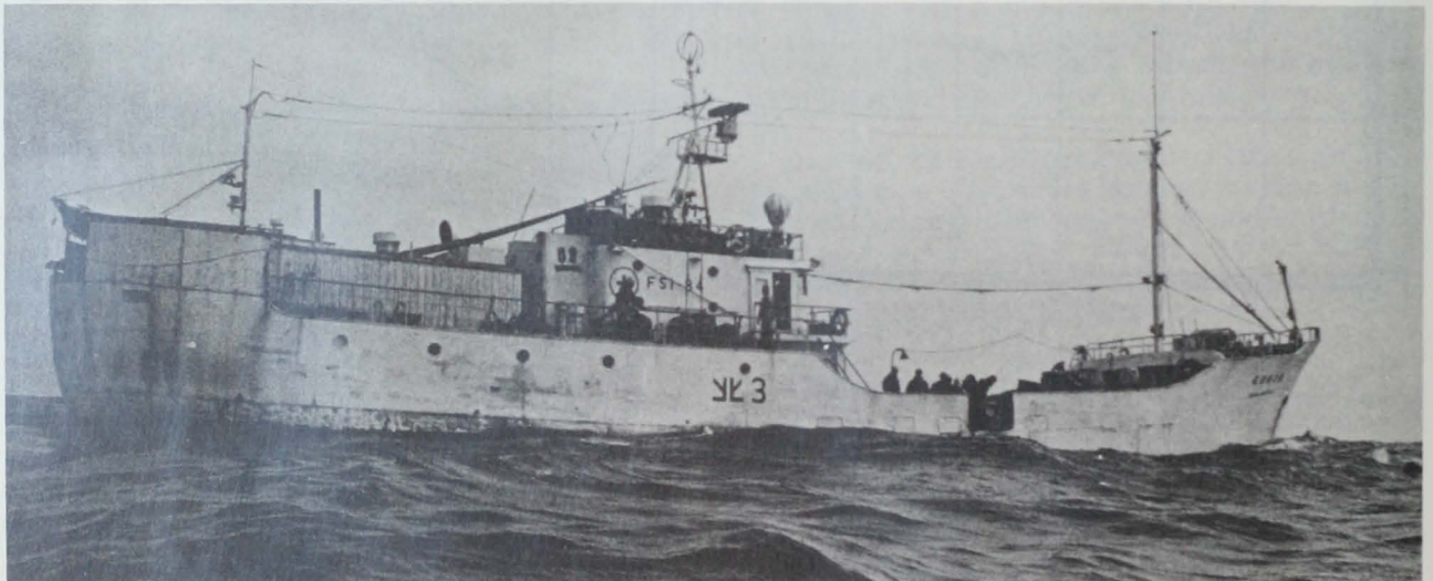
Fig. 2 - The longliner, 'Asahi Maru #7,' hauling gear in Gulf of Alaska. Typical of most longliners fishing sablefish off Alaska: machinery and crew spaces are aft, sharp-freeze compartments underneath the wheelhouse, and open working deck. Built in 1963, it is 192 gross tons, 128 feet long, powered by a 6 cylinder slow-speed diesel, and has a crew of 24. The baiting shelter is visible on the stem; so is opening from which gear is set.
