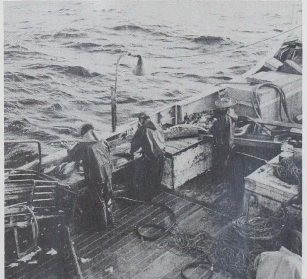
Fig. 5 - The butchering table on portside with gear-return chute visible on left. Fish are headed, eviscerated, and washed with sea water. Then they go down chute on right side into tub full of circulating water. From there they go either to a temporary storage bin or directly into freezer pans. Crew member on extreme right is untying at least 6 or 7 baskets of longline probably fouled during setting operation.
