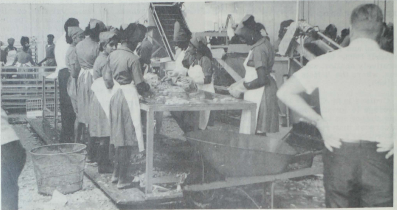
Fig. 1 - The processing plant of the American "Seafoods Guyana Company." Here, jumbo prawns are washed in chilled water. Then they are put in cardboard boxes and stored in cold chambers. Some lots are shelled to meet customers' requirements. Prawns are shipped to U.S. in a refrigerated ship.
