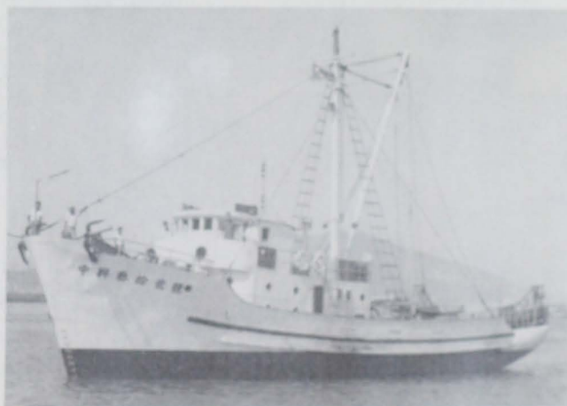
A full view of 'Chung Hsin 32,' a steel hull otter trawler of 150-ton class launched in August 1959.
