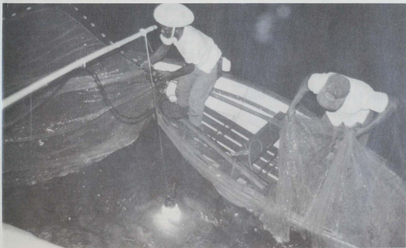
Fig. 4 - The UN vessels have tried live-bait fishing for tunny. To do this, the bait must be caught first. The vessels come into a different anchorage each evening and fish with a blanket net slung from outriggers.
