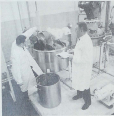
Fishburger is mixed with alcohol in unheated vessel to remove water and fats (they dissolve in alcohol).
