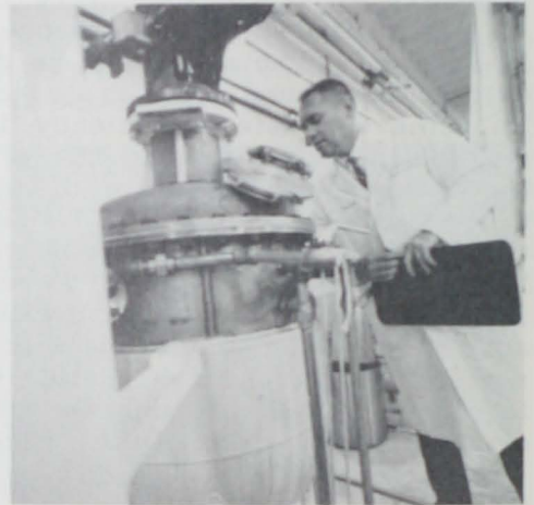
HOT ALCOHOL is used to continue the extraction of fats and moisture from the fish.
