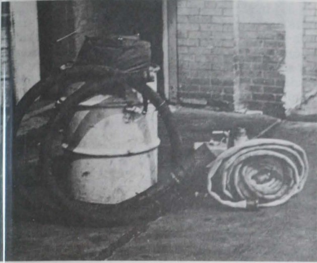
Fig. 12 - Emergency dewatering pump used by Search-and-Rescue Division of U. S. Coast Guard in assisting sinking fishing vessels. Gasoline-operated pump is packed in steel drum with intake and discharge hoses and lowered from helicopter or parachuted. (Photos 12, 14: J. J. Murray)
