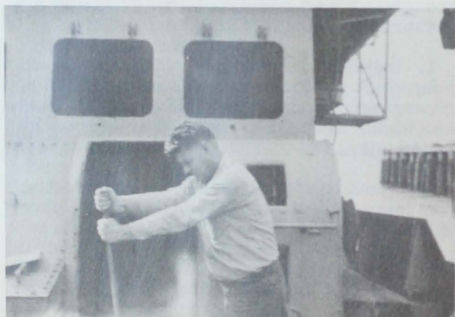
Fig. 4 - Hand steering wire on trawling winch, the cause of many injuries in otter trawling fleet.
