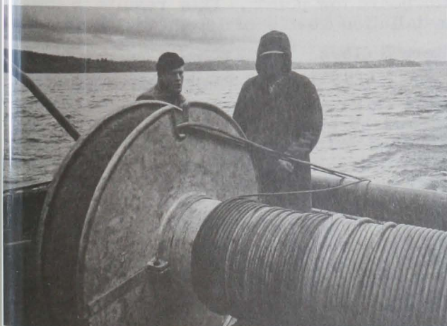
Fig. 2 - When the groundlines are nearly retrieved, they are pushed through a notch in the inner flange so that the trawl will be wrapped onto the center portion of the core.
