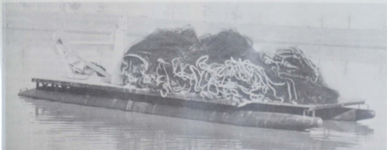
Fig. 2 - Nylon haul seine developed by BCF is stacked on pontoon barge and ready to set over stern roller. It is used in harvesting catfish from farm ponds.
