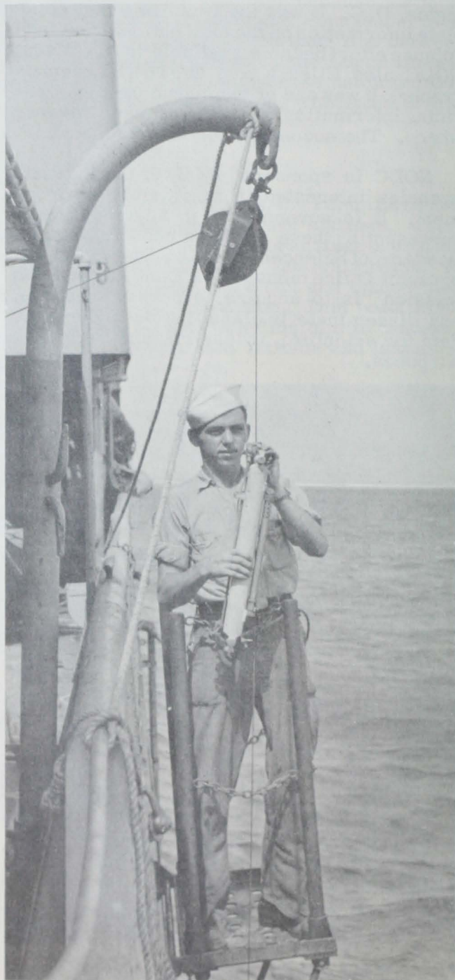
Fig. 4 - Nansen bottle is attached to wire to obtain temperature, pressure, and water sample at predetermined depth.
