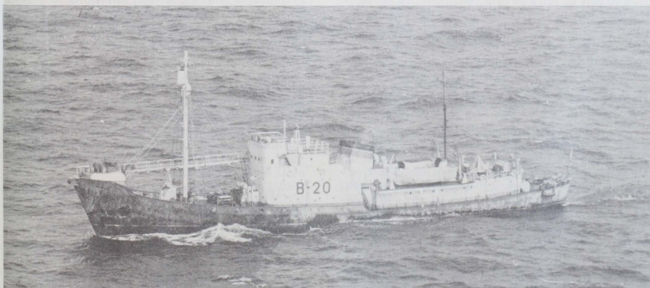
Fig. 1 - "Ryanyy," whale catcher. This type of vessel highly maneuverable and capable of 18-20 knots. It is 208 feet long. (BCF/Crosby)
