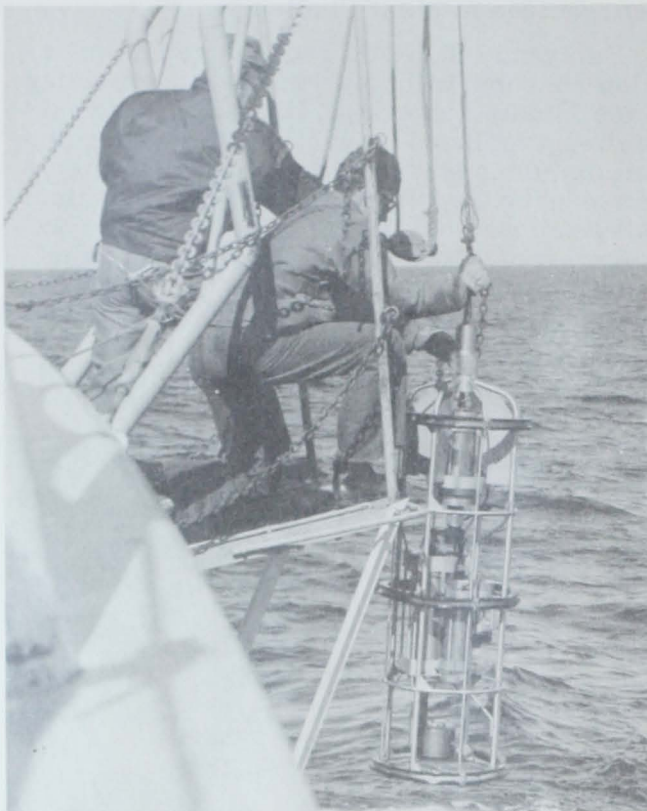
Fig. 3 - Ocean Science Important to Ice Patrol Vigilance--The constant study of the ocean currents, which greatly influence iceberg movements, is important to the Ice Patrol's predictions and tracking plots for iceberg seasons. Here, a Salinity Temperature Depth Sensor system is used on the Coast Guard oceanographic vessel "Evergreen" on a mission to determine if the source of the Labrador Current is in the Hudson Strait. The Sensor systems instantaneously record readings of salinity, temperature, and depths down to 1,500 meters. (U. S. Coast Guard)
