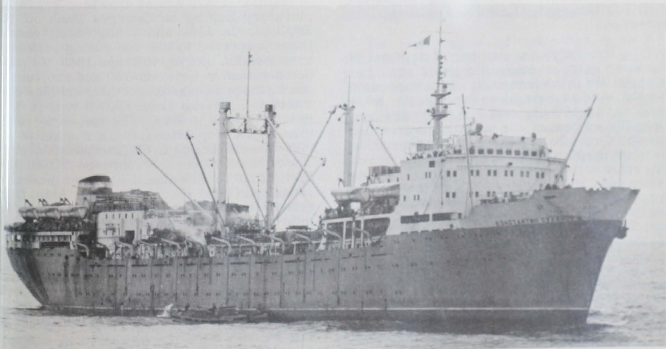
The "Konstantin Sukhanov," a passenger-freighter, was converted to a fish factory ship for crab fishing in the Bering Sea.
