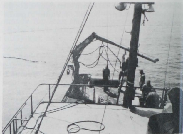
Fig. 3 - Retrieving 1,500 foot modified menhaden purse seine through power block aboard R/V Kaho.
