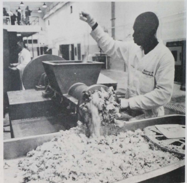
Fig. 1 - Red hake is dropped into grinder--producing, after water and fats are dissolved in alcohol, fish protein concentrate (FPC).
