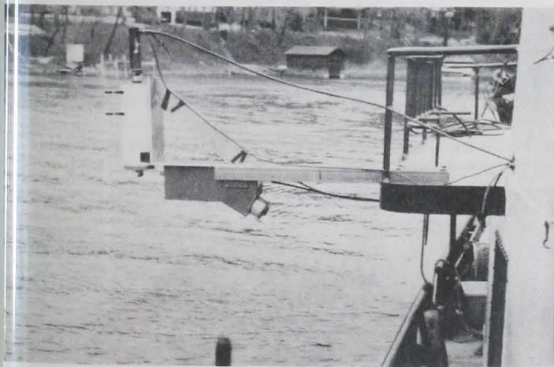
Fig. 1 - Compact LASER, optical transmitter and receiver, secured to the superstructure of the R/V Kaho.
