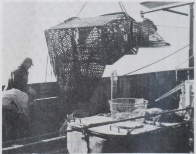
Fig. 5 - Modified 48-inch hydraulic dredge used during the 1965 surf clam surveys.
