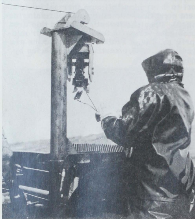
Fig. 2 - Experimental "auto-clips" connecting branchlines to the mainline were released by a prototype detaching device. When unattended, the detached clips were caught by the semicircular steel rake shown below the detaching mechanism.
