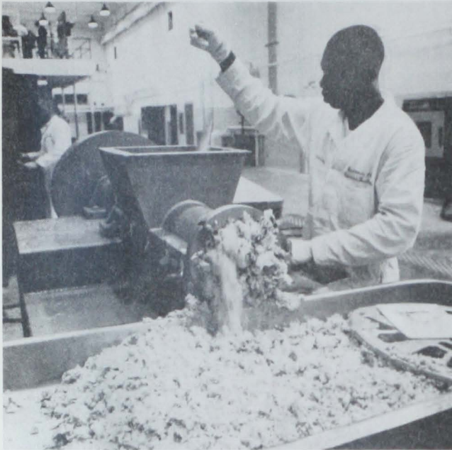
Fig. 3 - Red hake is dropped into grinder--producing, after water and fats are dissolved in alcohol, fish protein concentrate (FPC).
