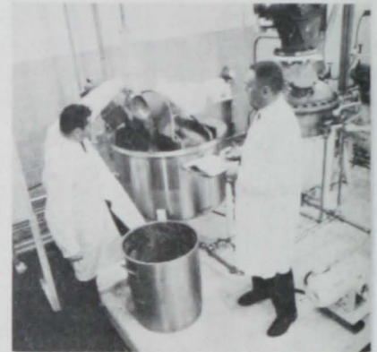
Fishburger is mixed with alcohol in unheated vessel to remove water and fats (they dissolve in alcohol).
