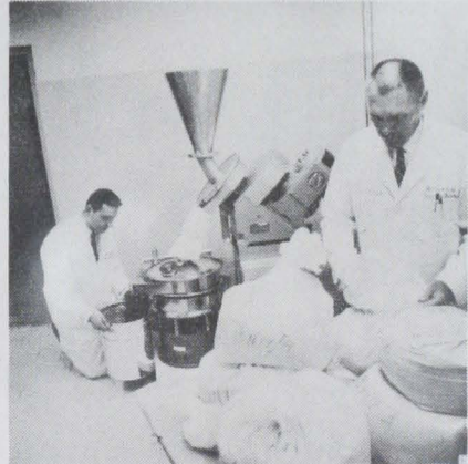
FINE GRINDER reduces fully dried FPC to particle size desired. It is bagged and marked to indicate the different experimental conditions under which it was produced.
