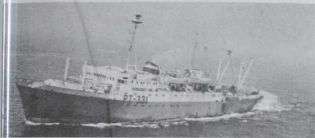
Fig. 1 - Soviet factory-type stem trawler fishing in the Northwest Atlantic.
