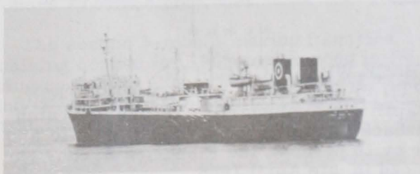
Fig. 1 - Japanese whale factoryship in Bering Sea. Note stern ramp for taking whale aboard.
