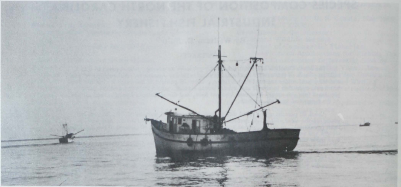
Fig. 1 - Double-rigged shrimp trawlers operating in coastal ocean waters near Beaufort Inlet, North Carolina.
