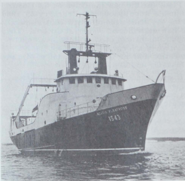
Fig. 2 - The Acadia Albatross , a modern Canadian stern trawler. The vessel, all-welded steel strengthened for navigation in ice, is 152 feet long overall. Vessel is operated by a Nova Scotia fisheries firm.
