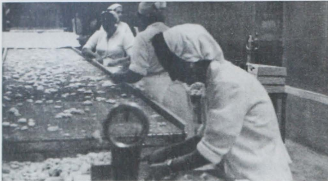
Breaded shrimp on conveyor belt moving to weighing and packaging line
