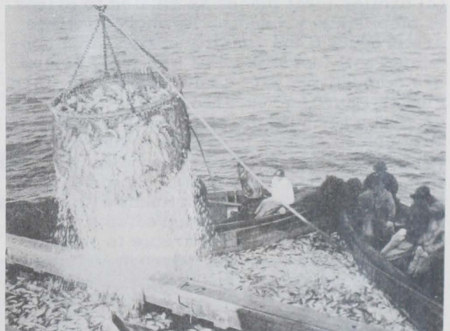
Brailing menhaden from the pocket or bunt of a purse seine. Fish meal, oil, and solubles are produced from menhaden. More modern purse seiners are now equipped with large suction hoses to transfer the fish from the net to the vessel.
